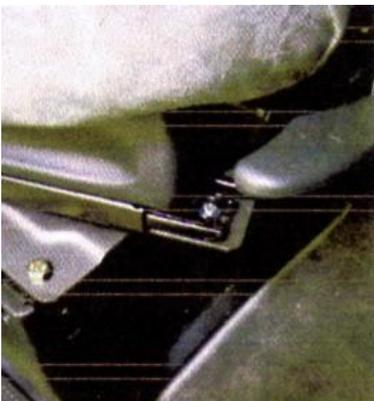
**6. Replace the seat on its base. This can be quite tricky so get someone to help you align the seat. Slide the seat back and pass one of the 8x20mm bolts up through the top part of the turntable and through the hole you've drilled in the rail, with the washers beneath and lock nut on the top. Repeat the operation, then slide the seat forward and fit the 15mm bolts to the back. Job done!**
